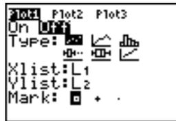
8. Press  $\boxed{ENTER}$  to select **On**, which turns on plot 1. Press  $\boxed{\downarrow}$   $\boxed{ENTER}$  to select  $\text{■}$  (scatter plot). Press  $\boxed{\downarrow}$   $\boxed{2nd}$   $\boxed{[L1]}$  to specify **Xlist:L1** for plot 1. Press  $\boxed{\downarrow}$   $\boxed{2nd}$   $\boxed{[L2]}$  to specify **Ylist:L2** for plot 1. Press  $\boxed{\downarrow}$   $\boxed{\rightarrow}$   $\boxed{ENTER}$  to select **+** as the **Mark** for each data point on the scatter plot.
