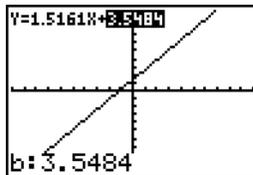
The screen dynamically displays the revised parameter value. Press  $\text{ENTER}$  to complete the modification of the selected parameter, save the value, and refresh the displayed graph. The system displays the revised parameter value in the symbolic expression  $Y=mX+B$ , and refreshes the graph with the updated Manual-Fit Line.
