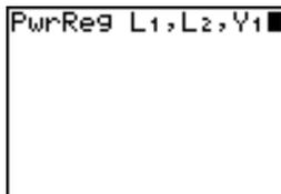
25. Press **[ENTER]** to calculate the power regression. Values for **a** and **b** are displayed on the home screen. The power regression equation is stored in **Y1**. Residuals are calculated and stored automatically in the list name **RESID**.
