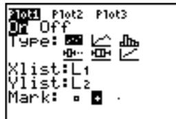
9. Press  $\boxed{ZOOM}$  **9** to select **9:ZoomStat** from the **ZOOM** menu. The window variables are adjusted automatically, and plot 1 is displayed. This is a scatter plot of the time-versus-length data.
