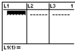
The top line displays list names. L1 through L6 are stored in columns 1 through 6 after a memory reset. The number of the current column is displayed in the top-right corner.
