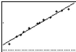
The regression line appears to fit the central portion of the scatter plot well. However, a residual plot may provide more information about this fit.
