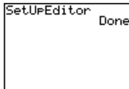
Press **[ENTER]**. This removes lists from stat list editor columns 1 through 20, and then stores lists **L1** through **L6** in columns 1 through 6.
