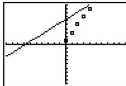
The linear function is displayed. The Manual-Fit Line equation displays in the form of  $Y=mX+b$ . The current value of the first parameter ( $m$ ) is highlighted in the symbolic expression.
